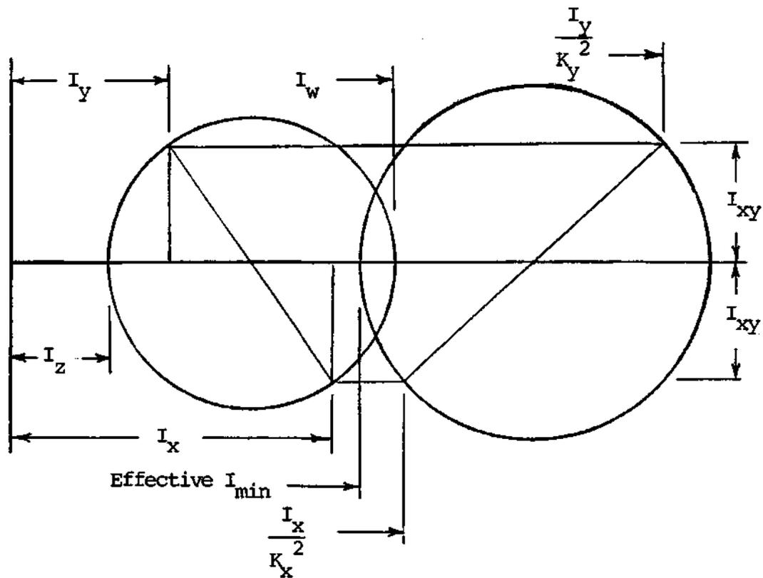
$$\text{Effective } I_{\min} = \frac{I_y}{2K_y^2} + \frac{I_x}{2K_x^2} - \sqrt{\left[ \frac{I_y}{2K_y^2} - \frac{I_x}{2K_x^2} \right]^2 + I_{xy}^2} \quad (8)$$
