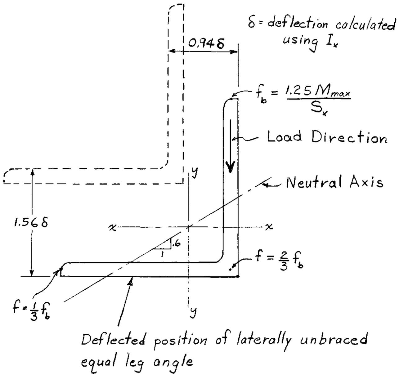
Figure 6 - Geometric Axis Bending of Equal Leg Angles
