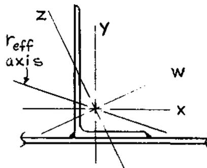
Figure 3 - Suggested Procedure for Effective Radius of Gyration
