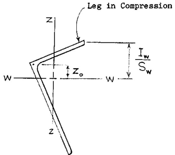
Figure 5 -  $F_{ob}$  for unequal leg angles bent about w-axis
